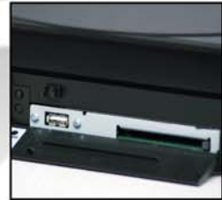
PCMCIA: Integrated PCMCIA and USB port in front. Part # 20300
